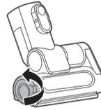
3. Wipe the inside clean with a cloth strip. If the roller brush is wrapped with hair, cut it along the roller brush with scissors and clean it up. After cleaning, mount the roller brush back according to the above disassembly steps.
