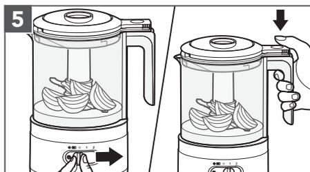
Slide the Speed Controller to your desired setting (1 or 2). Press down the Pulse/On Button to start.
