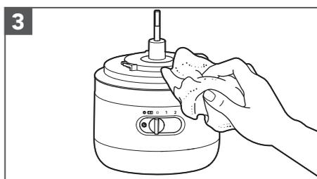
3 Wipe the Base with a damp cloth. Do not immerse the Base in water.
