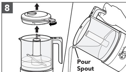
8 Once processing is complete, remove the Lid, Drive Adapter, and Multipurpose Blade to use the Pour Spout.
