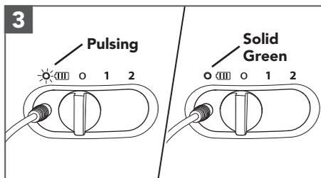
3 The Battery Status Indicator pulses when it charges. It will be fully charged in 2 hours and the Battery Status Indicator turns solid green.
