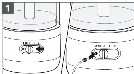
1 First, slide the Speed Controller to "0". Then, insert the Charger Adapter Pin into the Charging Port.
