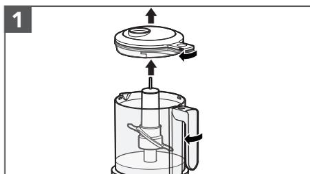
1 Remove the Lid, Multipurpose Blade, and Drive Adapter. Hold the Base steady. Twist and lift the Bowl to unlock from the Base.
