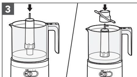
Rotate and lower the Drive Adapter and then Multipurpose Blade or optional Whisking Accessory in the centre of the Bowl until it rests at the bottom.
